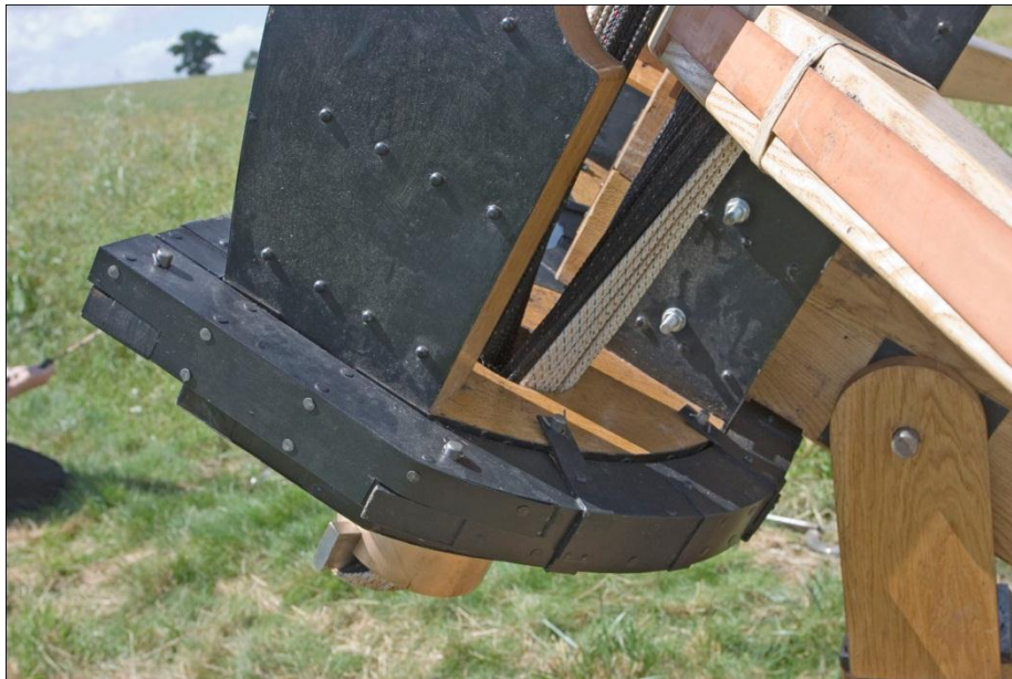
Fig. 12 : Details on the Mk I machine of one of the plated Crossbars joined to the ends of the Crossbeams by halving joints and pins. Also visible are the two metal straps which are Len's addition to secure the Crossbeams to the Hole-carriers, and the ends of the two bolts used as the Locking Bars.
