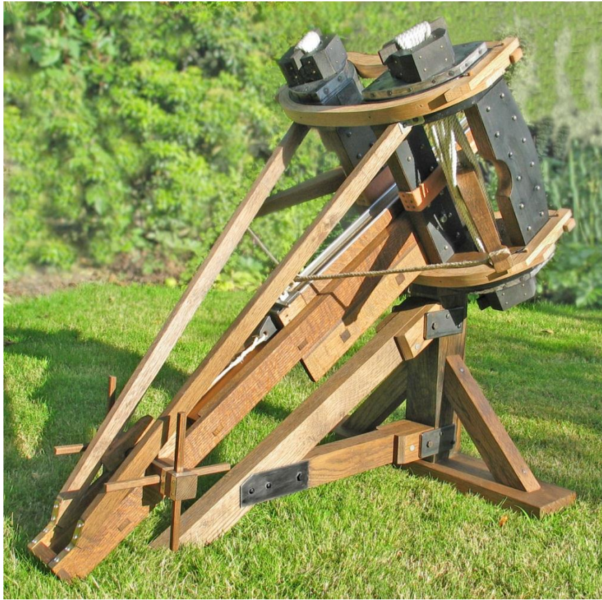
Fig. 18 : My large model (stock one metre long, scaled to a spring-hole diameter of 4.9 cm, 2 Roman inches) used as the basis for Len's full-size machine. It has the wooden Washers described by Vitruvius and Heron (p. 7-8 and figure 5). I have also added Philon's thick counter-plates under the Washers (Appendix 2 for corrected reading of his text): he gives their thickness as one quarter of the diameter of the spring-hole, too thick for them to be cast in metal, so I have presumed them to be plated blocks of wood. They are not mentioned by Vitruvius, and are omitted on our Mk I version. The bowstring on the model is far too narrow, and there is room for a lot more spring-cord.
