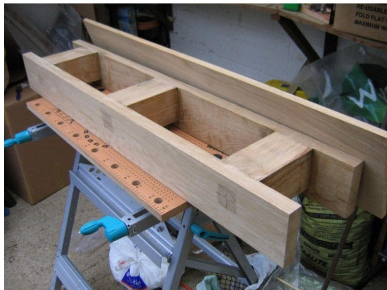
Fig. 19 : Len’s Table, with the plank ready for fastening on top of the sides and cross-struts (photo : Len Morgan).
