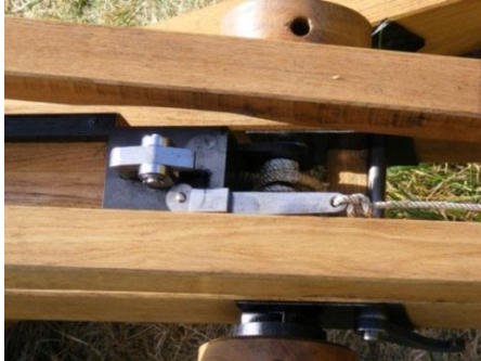
Fig. 23 : (left) Looking down between the two Stays onto the Trigger. Its release lever is in the released position, having been operated by a long rope from several metres behind the catapult for safety reasons. (right) Side view of the Trigger and its mounting plate. (photos : Len Morgan)
