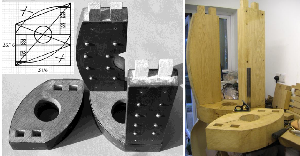
Figure 2: Left: The writer's model of a Half-spring frame, scaled to a Spring-hole diameter of 2 Roman unciae (4.9 cm), based on the following interpretation of Vitruvius' rhombus figure. The plating described by Heron has been added. Right: Len Morgan's photo of his oak frame under construction to Vitruvius' 2 librae size, with a Spring-hole diameter of 5 Roman unciae (12.3 cm). The semi-circular cutout for the arm in the Side-stanchion has not yet been made. The position of the tenons on the inner face of the stanchions is based on the evidence of Heron's rhombus diagram in figure 4.
