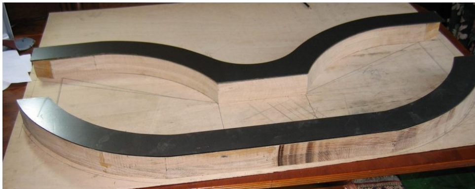
Fig. 11 : Len's Crossbeams with top plating. The straightened central part of the Outer Crossbeam helps to maintain the spacing between the two Hole-carriers. (photo: Len Morgan)
