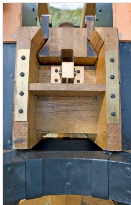
Fig. 21 : Realisation by Len of my interpretation of the cross-section of Table, Ladder and Slider. Note (left) the bracket and spindle holding the pulley wheel feeding the windlass rope from the Central Gap under the Ladder's Inner Beams to the channel in the base of the Slider.
