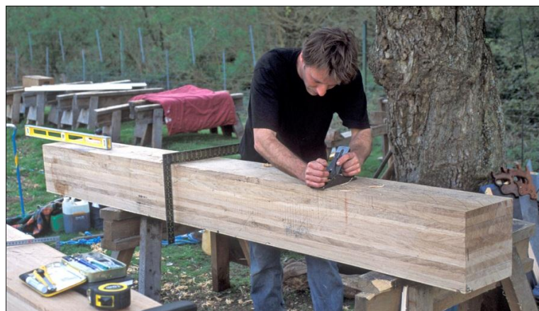
Fig. 27 : Starting to shape the huge arm for the BBC's One Talent (26 kg) ballista , using horizontally laminated ash.
