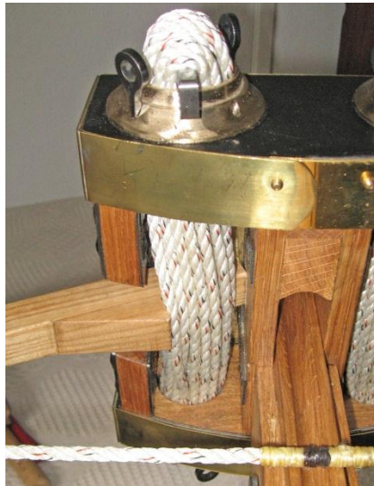
Fig. 4 The mistake in drilling the spring-holes off-centre, which will lead to spring-rope wear.
