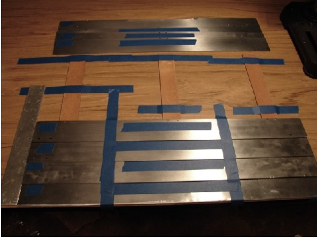
Halfway through the layout of the left girdle plates. Use a drill bit and turn by hand through the holes in the top of each plate to mark the positions in the straps.
