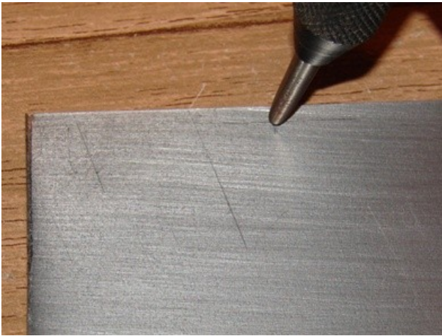
Using a spring loaded center punch to mark the location to drill (scratch marks exaggerated)
