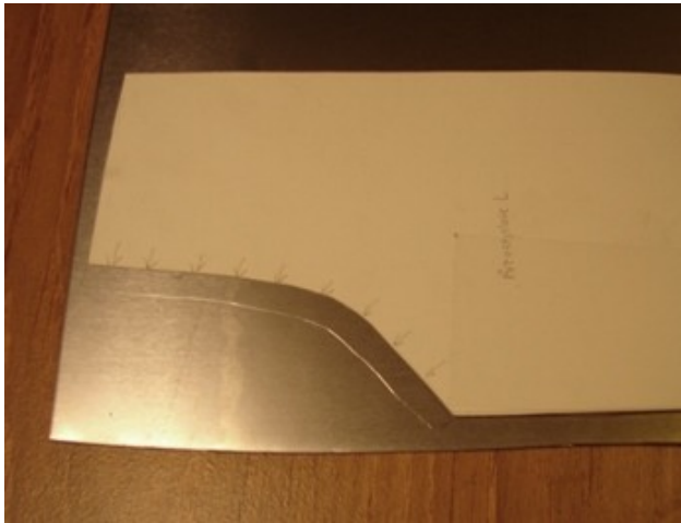
Tracing a pattern onto the sheet steel--note the score mark in the above pattern showing the allowance for the flared edge.
