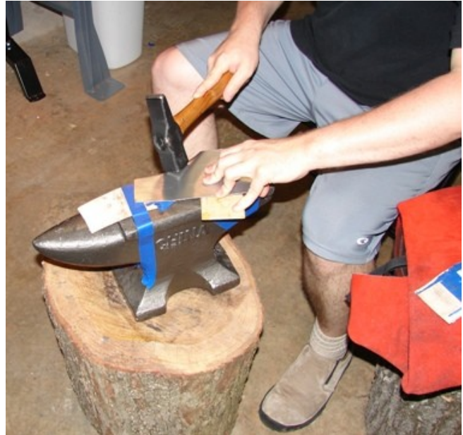
Using a hammer to bend the flared edge on the breastplate. Notice the wood plank supporting the plate at an angle on the anvil.
