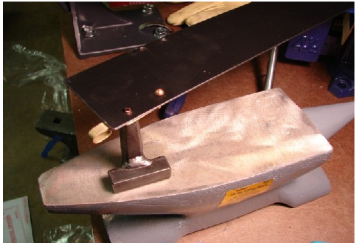
The rivet on the left is about to be peened. The one on the right is simply there to keep the fitting from moving around.
