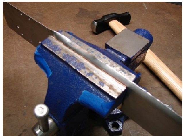
2. Starting the second pass. Bend over about another 45 degrees.
